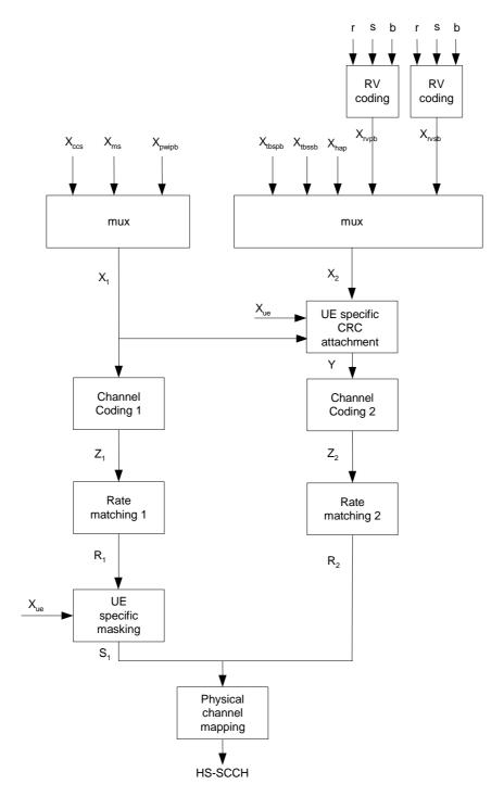
Figure 19B: Coding chain for HS-SCCH type 3
